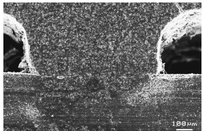
Fig. 7. SEM micrograph of cross-section of sintered ceramic sample showing good bonding between layers.
